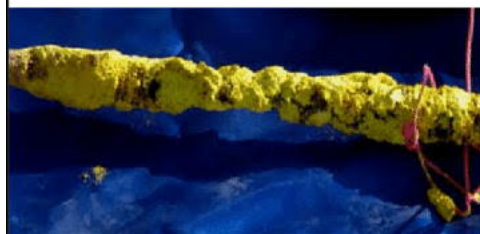
Weathered, unfired, rod with yellow uranyl salt deposits
